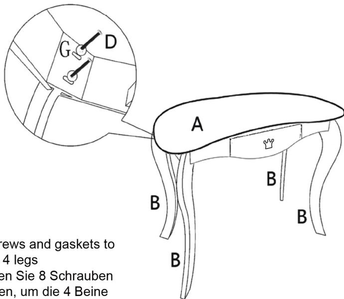
EN: Use 8 screws and gaskets to assemble the 4 legs
